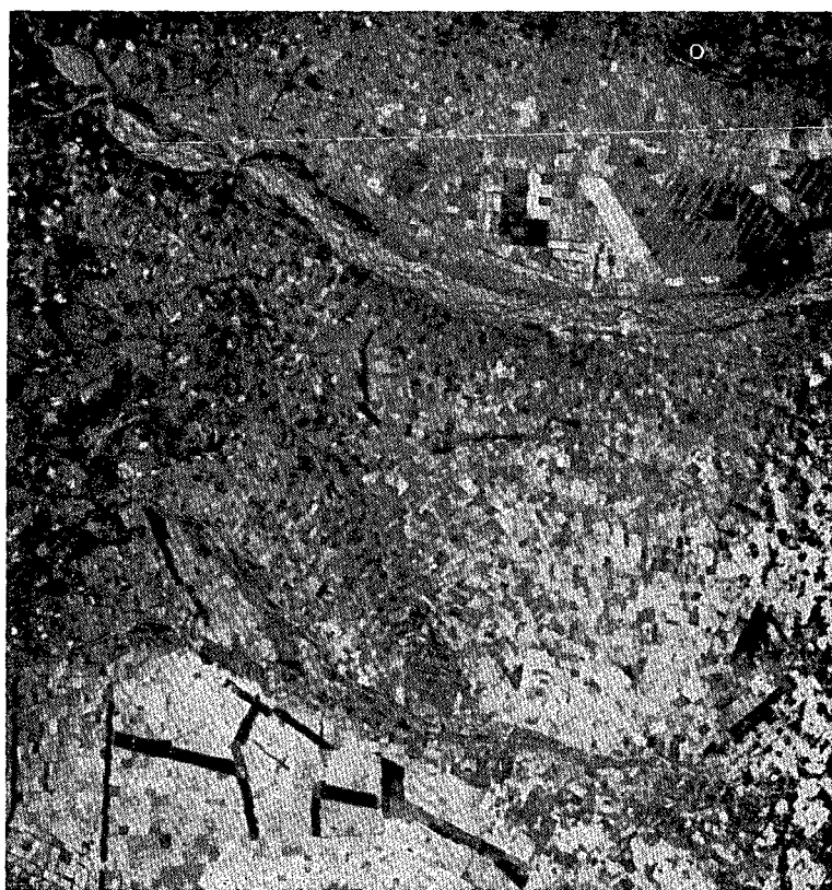
FIG. 3: MSS band 5 enlargement of mid-Canterberry region around the Waimakariri River. Note the pine shelterbelts (dark bands) near Darfield and south of the Selwyn River. Roads and river channels can be clearly seen on this photowrite enhanced product derived from numerical (CCT) data. Part of the scene shown in Fig. 2.
