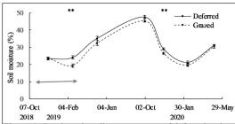
Figure 4 Gravimetric soil water content of deferred and grazed pastures at a depth of 0–7.5 cm averaged over 6 paddocks on 3 farms in Waikato / Bay of Plenty. Error bars represent the standard error of difference. The arrow denotes the grazing exclusion period in the deferred treatment. Asterisks denote when differences between treatments are significant: \*\* P<0.01.
