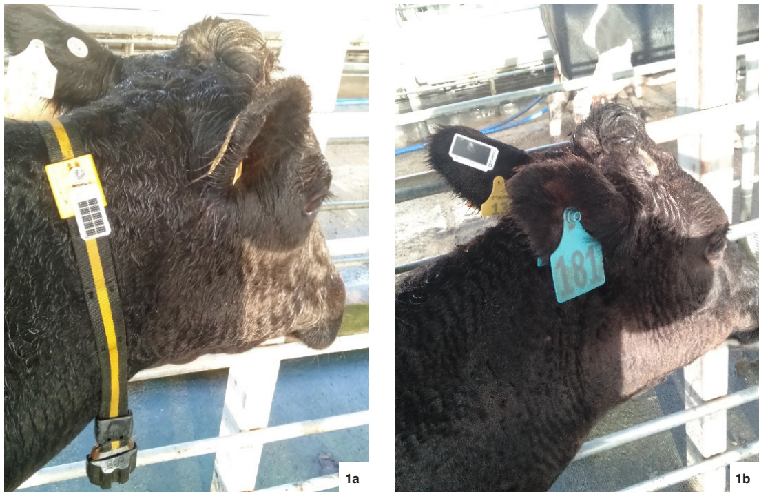
Figure 1 GPS devices on dairy cows during the trial period. Photo (a) on the left shows a GSatSolar ear tag attached to a cow collar, while photo (b) on the right displays a Ceres Trace ear tag (white rectangle).
